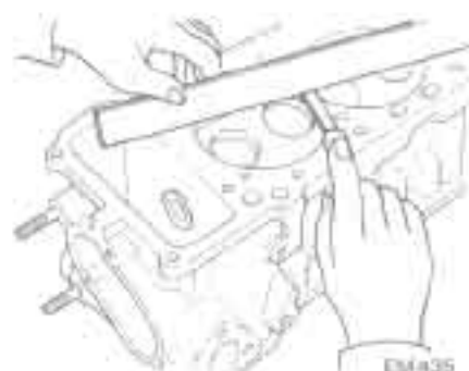
Fig. EM-30 Checking cylinder head surface
