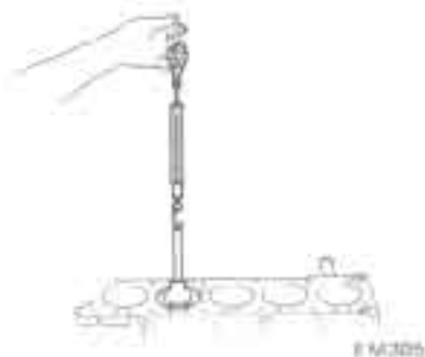
Fig. EM-51 Measuring piston fit in cylinder
