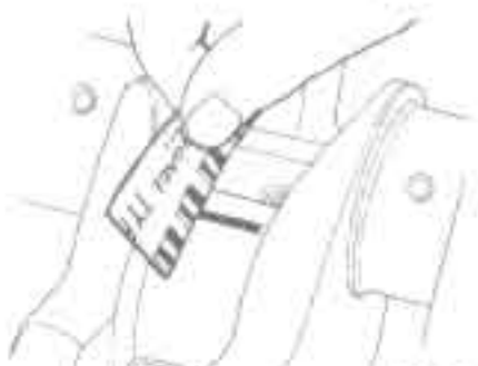
Fig. EM-64 Measuring bearing clearance
