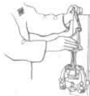
Fig. EM-56 Checking rod alignment
