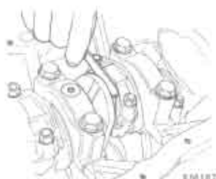
Fig. EM-95. Checking big end play
