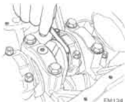
Fig. EM-57 Checking big end play
